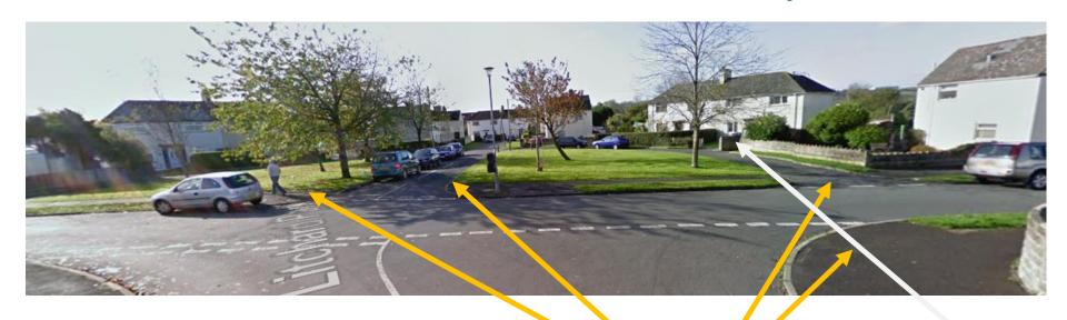
At the intersection between Litchard Park and Pendre a dropped kerb and tactile paving crossing is required to enable safe crossing of the road and onwards to the community centre (polling station) and Great Western Avenue Playing fields. Further tactile paving will be required as the pavement crosses the Pendre crescent
