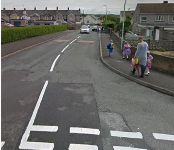
The route proceeds along Garfield Avenue and follows the continuous pavement into an unnamed road. Again the pavement is in good order at this point although a dedicated crossing point with dropped kerbs and tactile paving could be installed at this point to enable safe access eastwards along Garfield Avenue and onwards to Litchard Hill.
