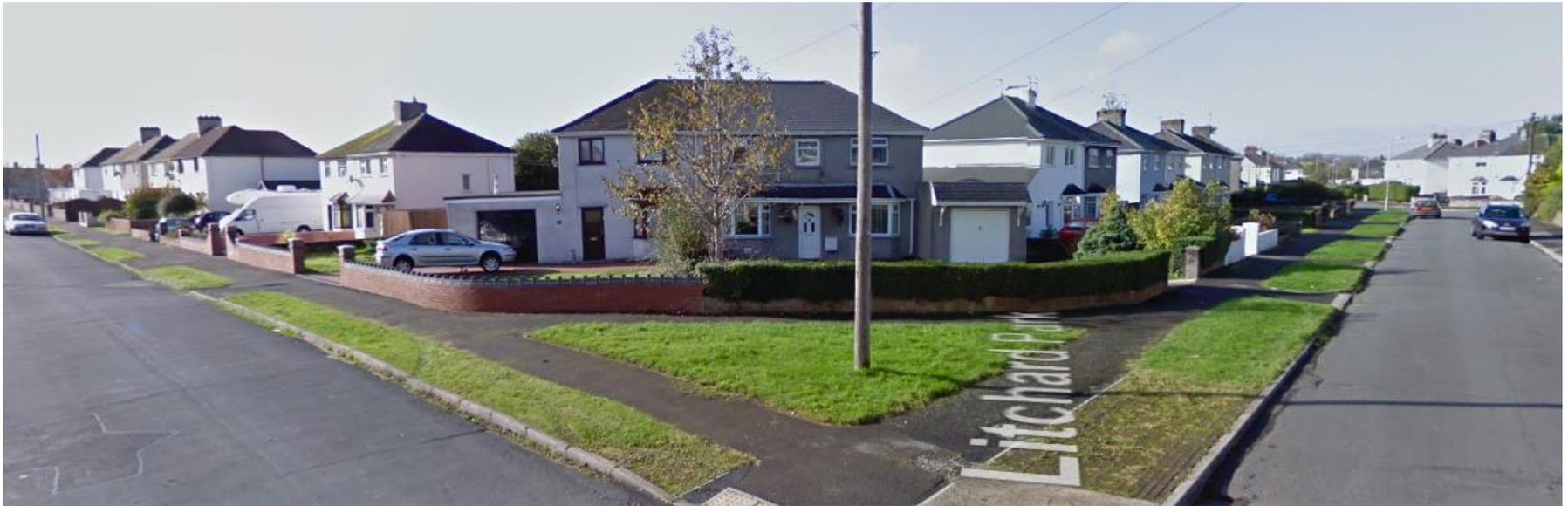
The pavement along Litchard Park as it progresses along Route 2 towards Pendre is in good order and suitable for incorporation into the active travel route. Although as Litchard Park heads eastwards towards Coity Road the tactile paving is inadequate and will need to be upgraded.
